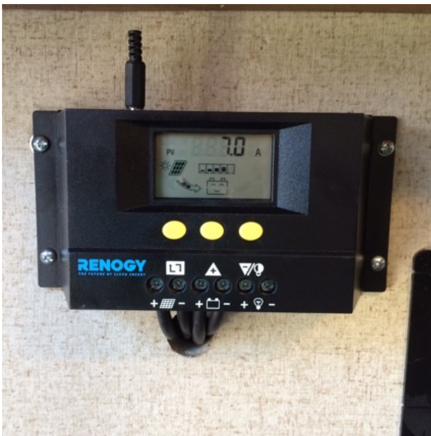
Full sun at around 12PM, noon, the panels are putting out 7.0 Amps, the max that can be expected.
