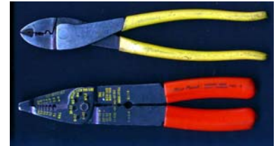
NOT RECOMMENDED CAN'T DO A GAS TIGHT CRIMP
